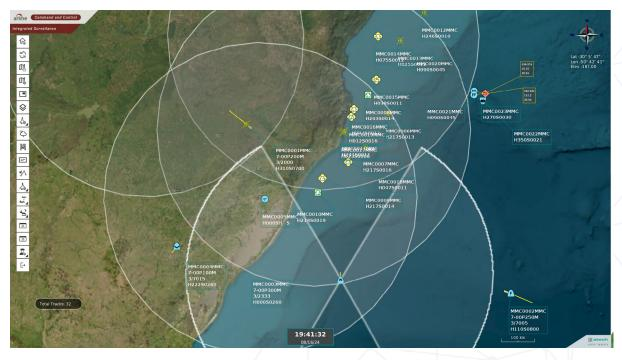
System HMI, geolocation of contacts, tracks, and targets.
